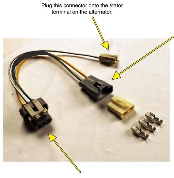
If you have an American Autowire (AAW) harness that comes with an "SI" series, internally regulated alternator connector, simply plug that alternator connector into this adapter. The "SI" series alternator connector is a white connector wired with a brown and a red wire.
